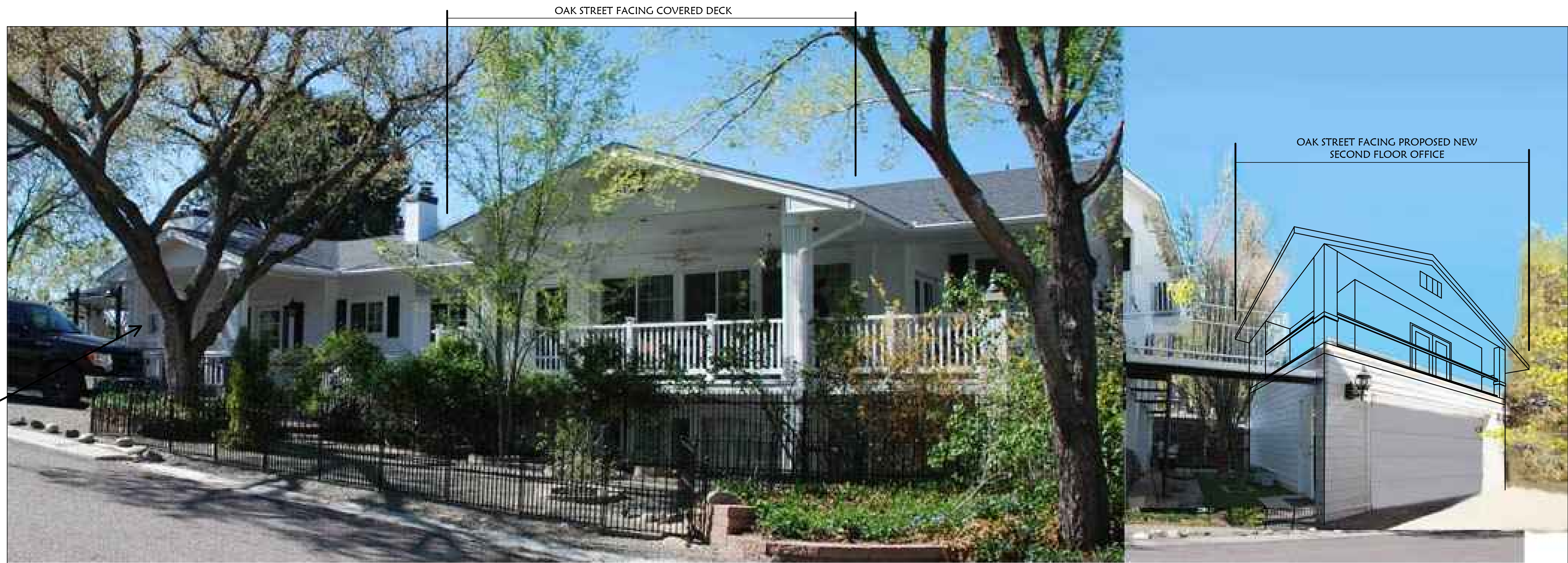
EXISTING OAK STREET ELEVATION OF DONOHUE-MALZO RESIDENCE SHOWING SUPER-IMPOSITION OF NEW SECOND STORY OFFICE OVER EXISTING GARAGE
