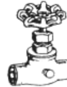
Stop & Waste Valve
